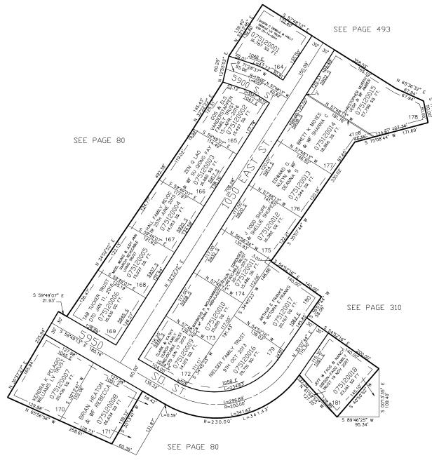
10' UTILITY & DRAINAGE EASEMENTS EACH SIDE OF PROPERTY LINES AS INDICATED BY DASHED LINES EXCEPT AS OTHERWISE SHOWN.
